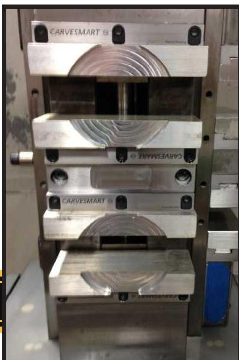
**“** We can change all 16 jaws on our quads in 10 minutes. We recut the female form to perfectly match the jaws to the spindle and are making good parts in half an hour instead of half a day. CARVESMART™ is now on most of our vises and the guys love it. **”**
